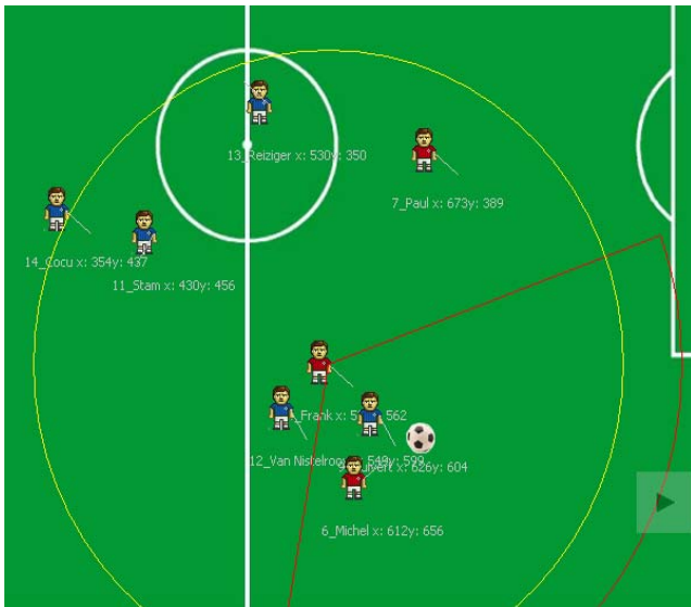
Figure 3. Part of the soccer simulator. The yellow circle defines the shouting distance, red arc is what the player sees
